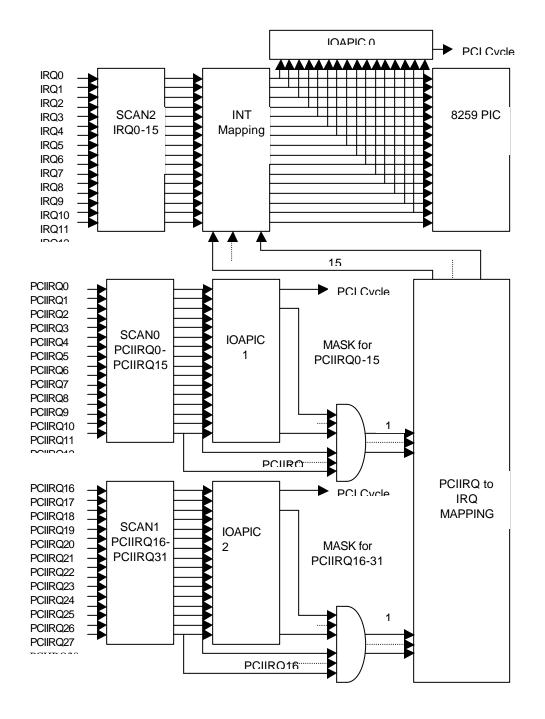
Figure 3. SDS2 Interrupt Routing Diagram (CSB5 Internal)
